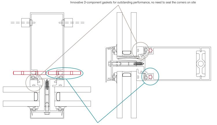
Smart pins system for fast and easy installation, loads up to 400 kg
